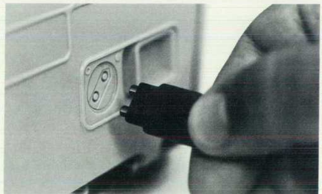
Fig. 3. A novel key can be used to lock the door to the card cage.
