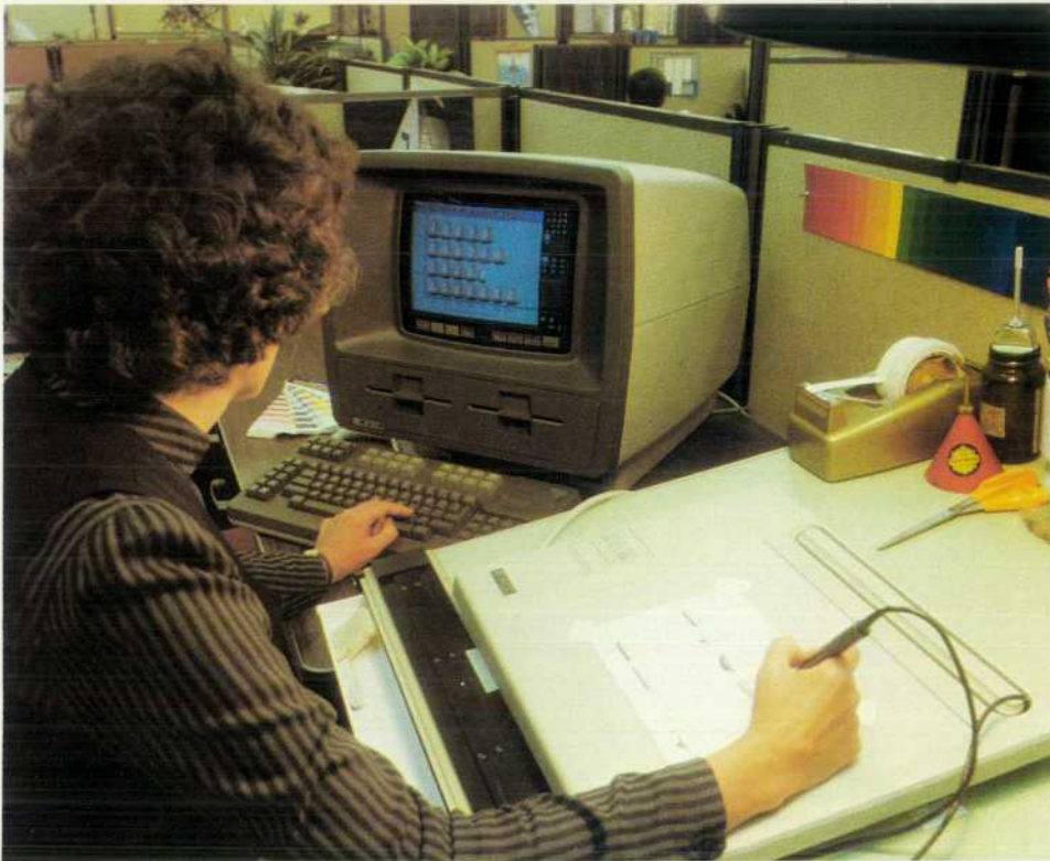
Fig. 1. The HP 2700 Color Graphics Workstation speeds the preparation of high-quality presentation graphics. The designer works with a keyboard, thumbwheels and a button, or an optional graphics tablet.
